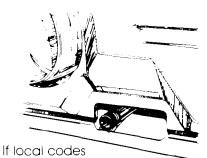
■ permit, it is recommended that flexible metal tubing be used for connecting the appliance to the gas supply line. (The gas pipe which extends through the lower rear of the appliance has ¾ inch male pipe thread.)
